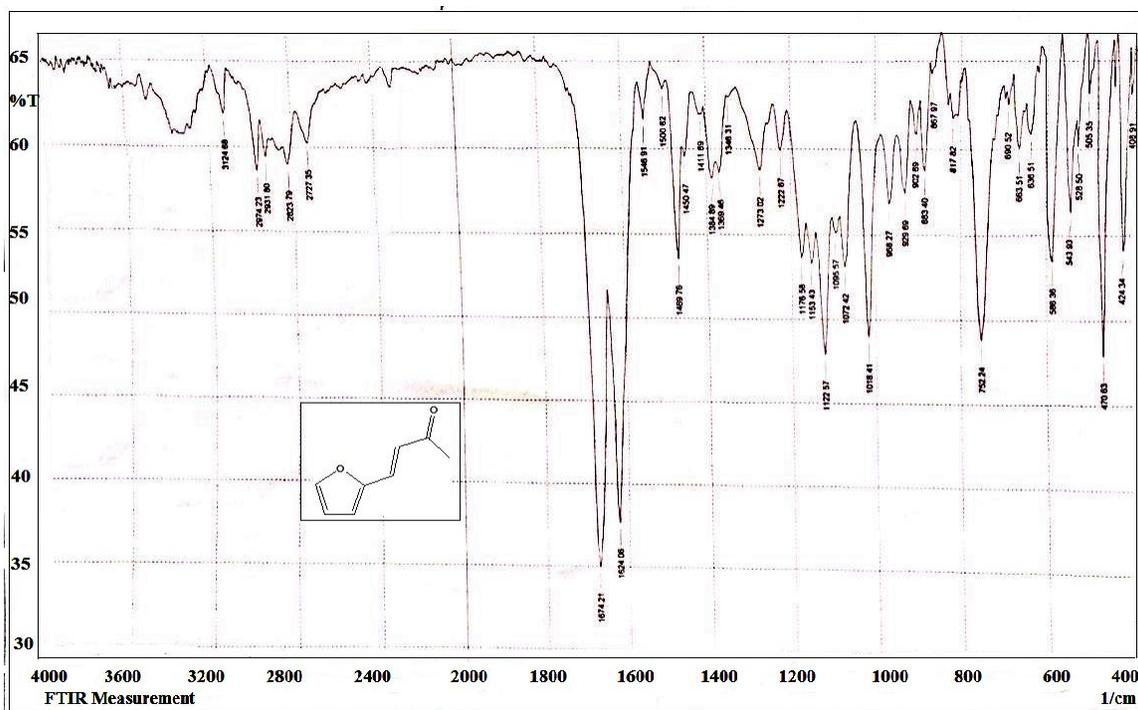
Figure 3-3: FTIR Spectrum of compound [3]
