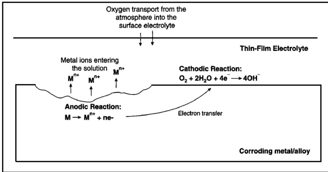
Figure 1-24: Schematic diagram of corrosion cells on metal
