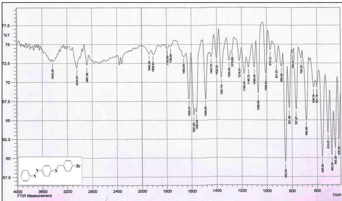
Figure 3-5: FTIR Spectrum of compound [5]
