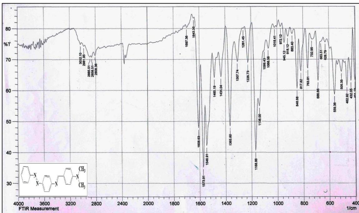
Figure 3-4: FTIR Spectrum of compound [4]
