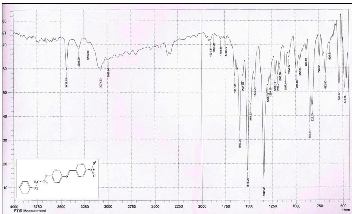
Figure 3-51: FTIR spectrum of compound [20]
