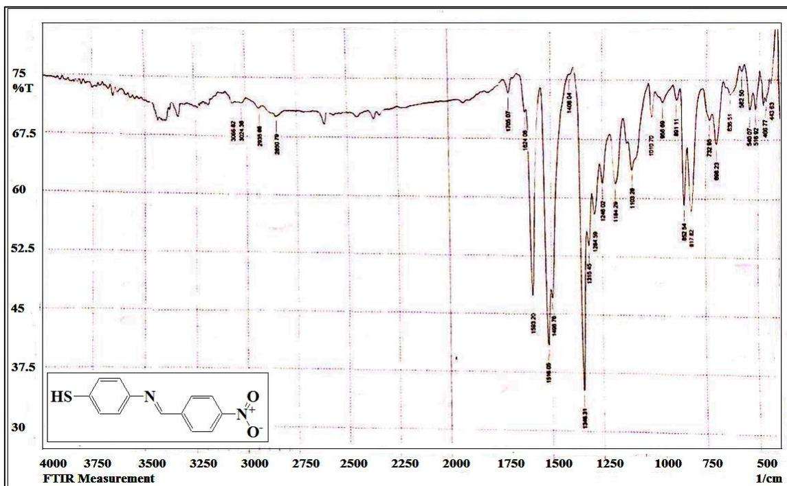
Figure 3-32: FTIR Spectrum of compound [12]
