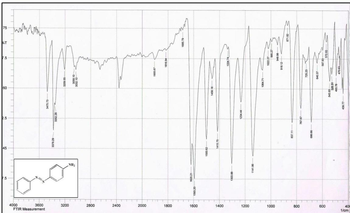
Figure 3-1: FTIR spectrum of compound [1]
