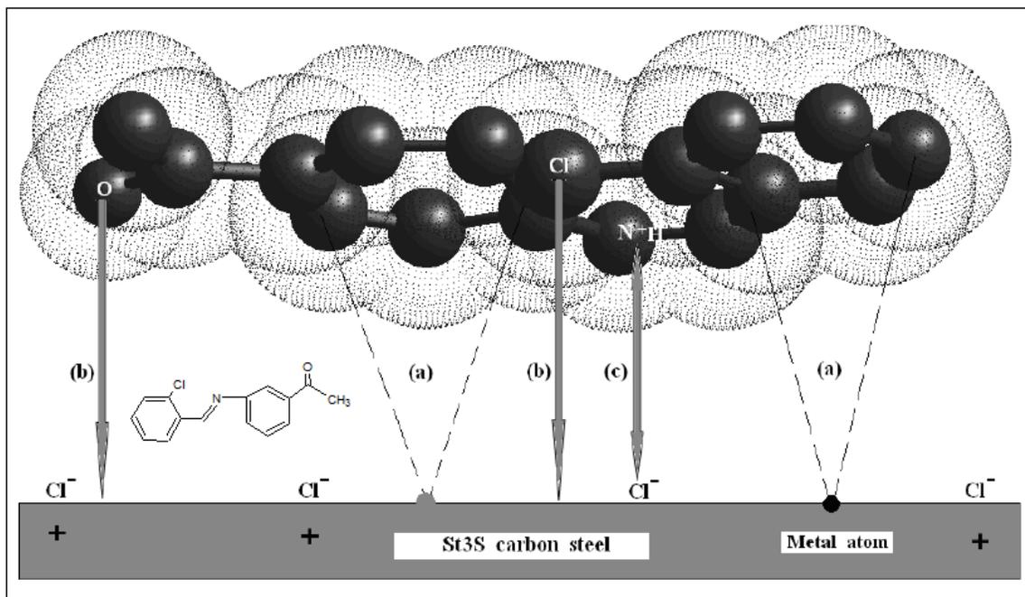
Figure 1-18: Proposal of model of protective layer of (CBAA) on St<sub>3</sub>S surface in a 1.2 M Cl<sup>-</sup> solution: (a) chemisorptions, (b) feedback bond, and (c) electrostatic interaction (physisorption)
