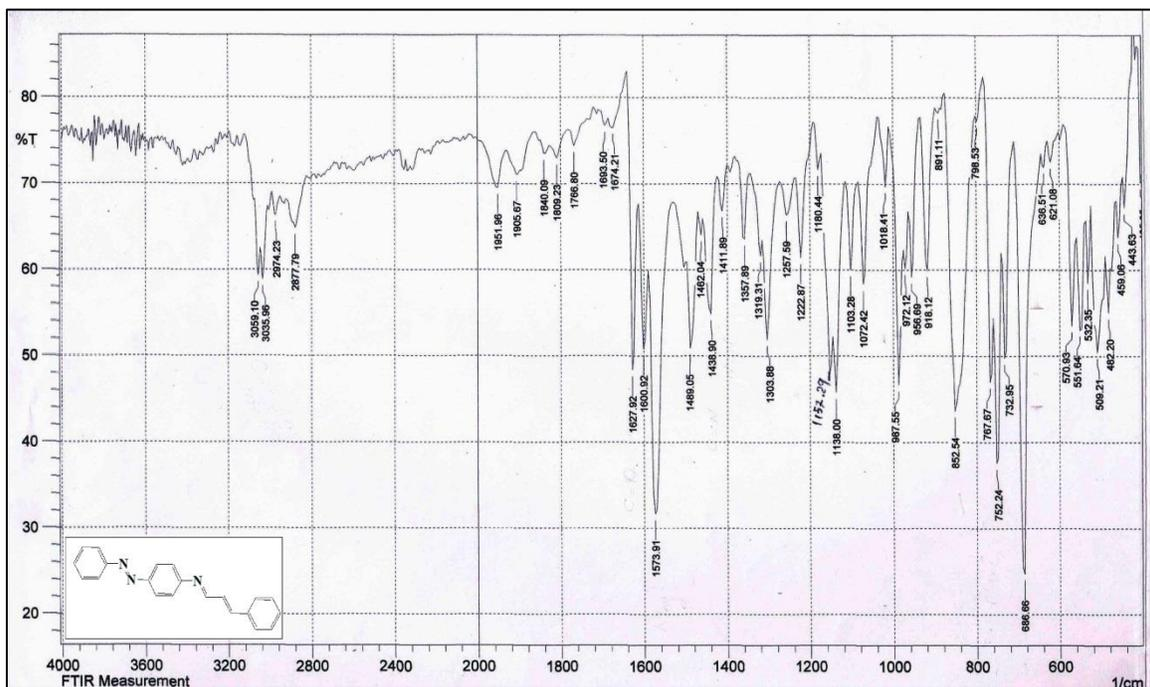
Figure 3-9: FTIR Spectrum of compound [9]
