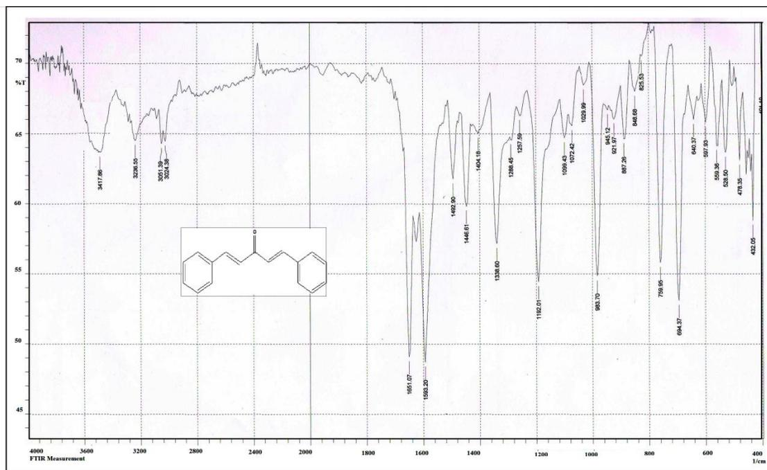
Figure3-2: FTIR Spectrum of compound [2]
