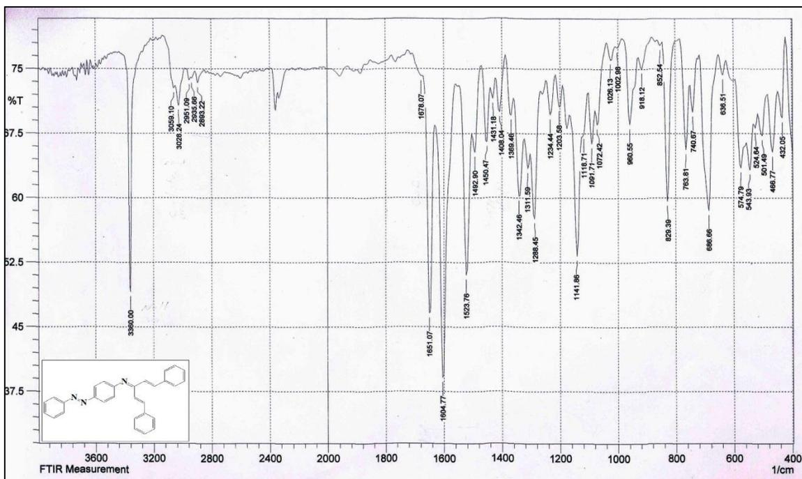
Figure 3-8: FTIR Spectrum of compound [8]
