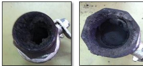
**Figure 5-33** Blockages in the outer tubes of the gasifier
