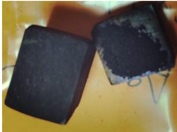
Figure.3.11: Fracture surfaces of graphite – stainless steel
