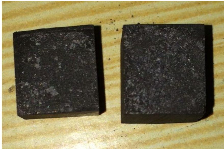
Figure 3.10: Thin layer of filler metal on the two samples of graphite.
