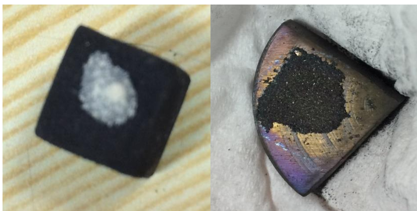
Figure 3.6: The wettability of titanium on both graphite and stainless steel.
