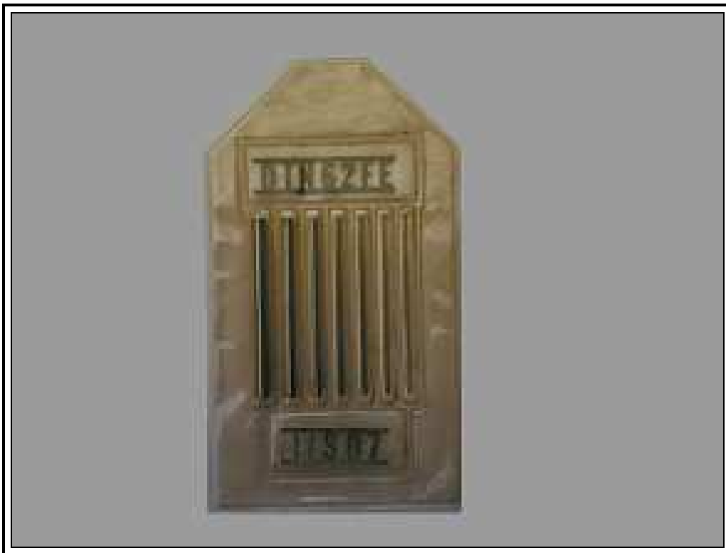
Fig. (2.7) A photograph illustrates wire type penetrameter
