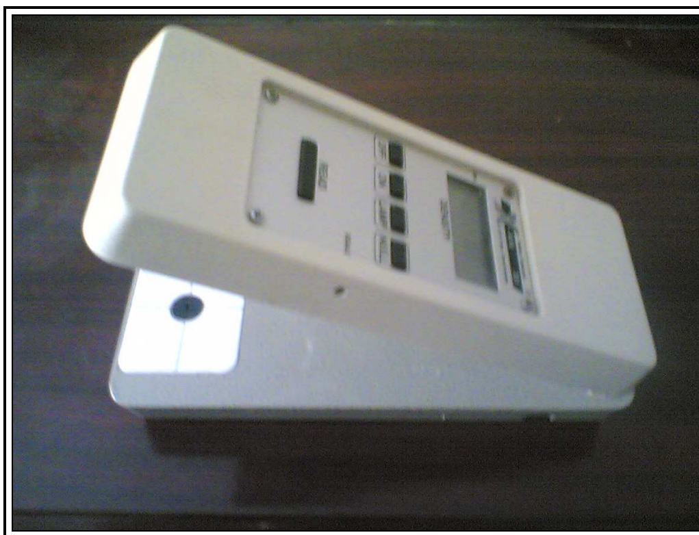
Fig. (2.6) A photograph illustrates a transmission densitometer (Grandvill,Michigan)used in this work
