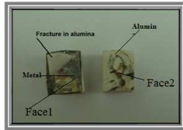
Fig. (3.9) The fracture in alumina part for Ag sample
