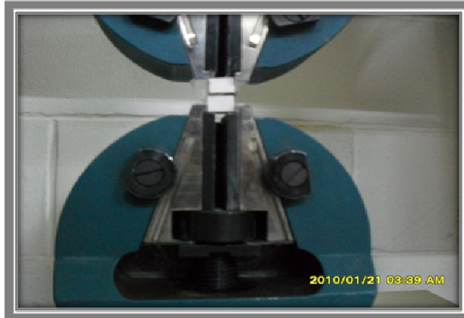
Fig. (2.5) Joining sample under test.
