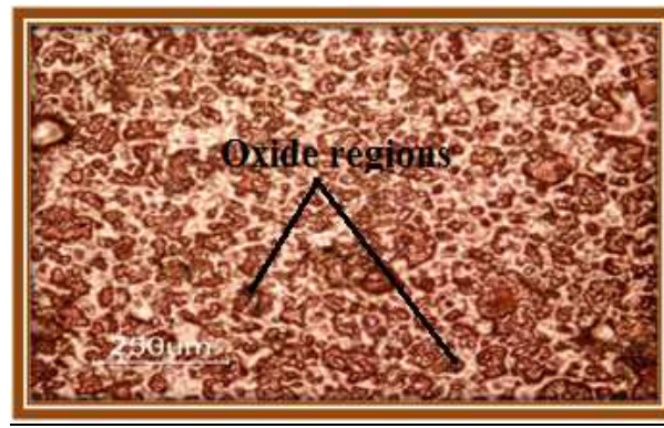
Fig.(3.29) optical Microscope image for face1 for Copper. (Magnification 100x )
