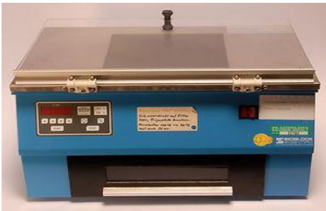
Figure 2.3 Vilber Lourmat FLX-20M Transilluminator 312/254 nm UV-irradiation system model and the amount of power 15W, the uv-radiation range was 1 J/cm 2 to 360 J/cm 2 , this system is located in the department of bio-technology in the college of science / Al-Nahrain university
