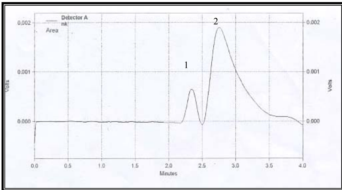
Figure (3-5). Chromatogram of polyaromatic compounds 0.5ppm phenanthrene(1) 1ppm acenaphthylene (2), with new packed column using mixture of hexane and isopropanol (40%,60%) as mobile phase, flow rate 1ml/min. detection wavelength 254nm.
