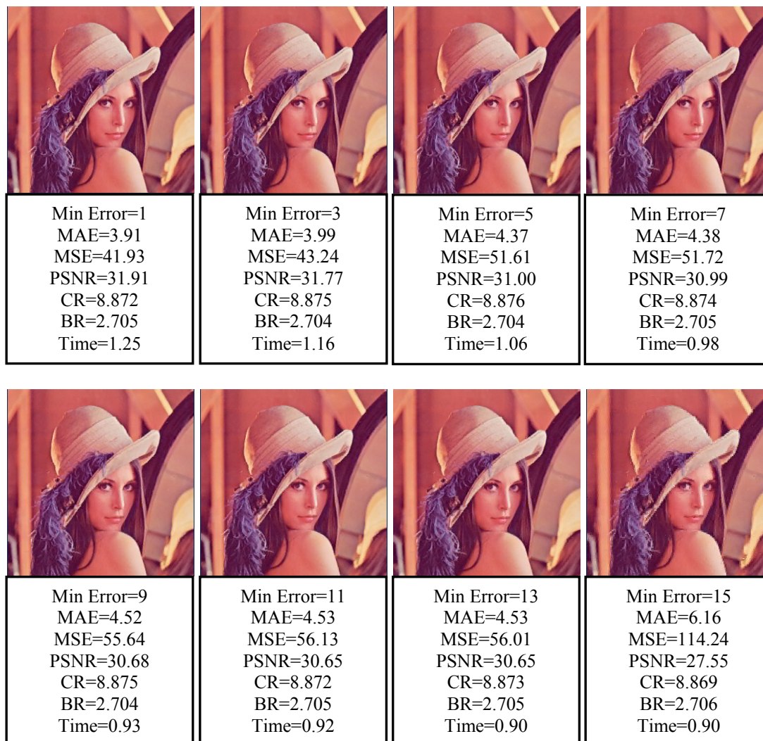
Figure (4.16) Samples of the reconstructed Lena image when it is compressed by Dis1FIC scheme using different values of minimum error
