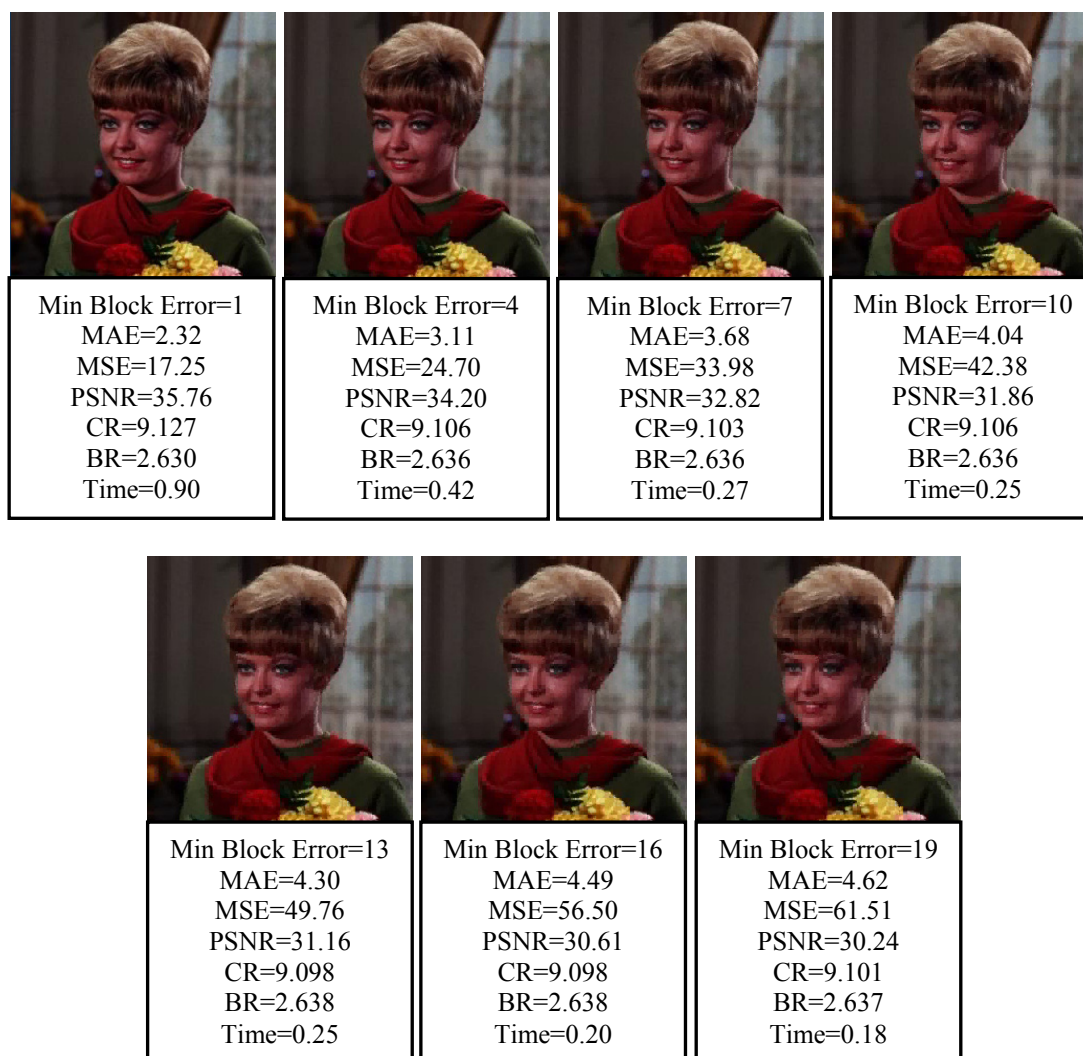
Figure (4.20) Some samples of the reconstructed Girl image when it is compressed by Dis1FIC using different values of the parameter "minimum block error"
