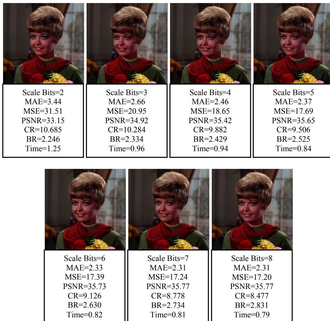
Figure (4.10) Some samples of reconstructed Girl images when it is compressed by Dis1FIC using different values of scale bit parameter
