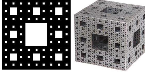
Fig.(4.1) The Sierpinski carpet (pores in white) and the Menger sponge (pores in black) [56].
