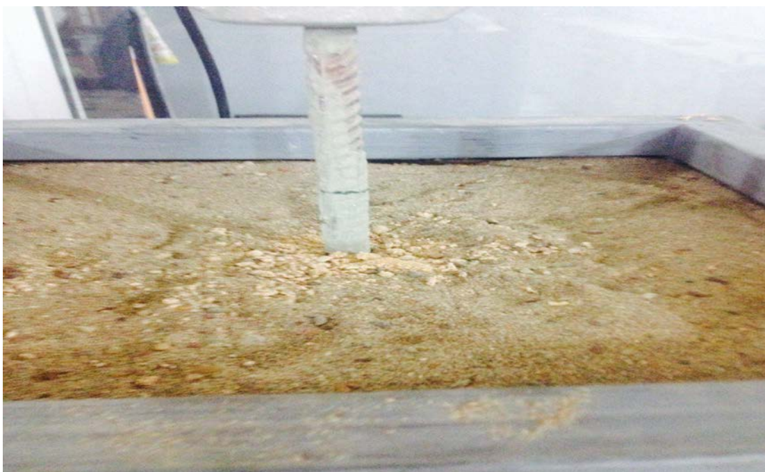
Figure (4-14). Bored pile model test
