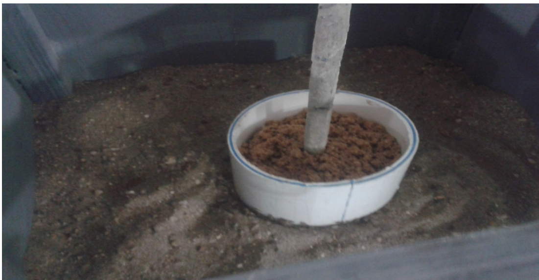
Figure (4-13). Bored pile model installation
