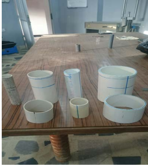
Figure (3-15). Casing pipe using in case of improving surrounding soil (bored –driven)
