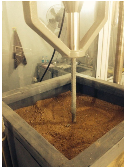
Figure (3-13). Bored pile model installation
