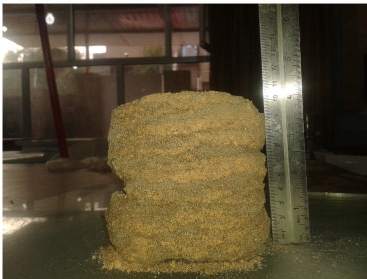
Figure (4-26). Soil block in bored case keep it structure constant approximately
