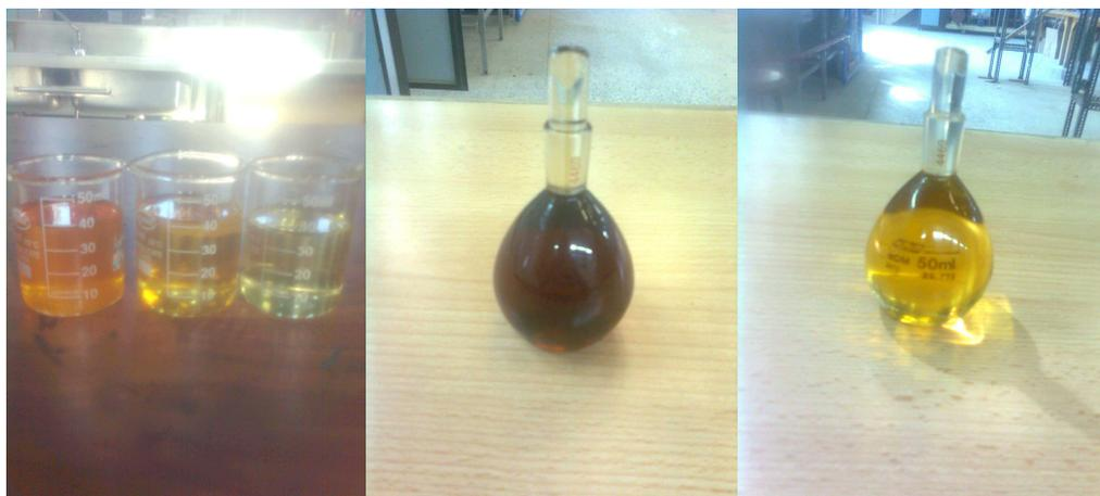
**Figure 5.6** Effect of changing the temperature on color of product.
