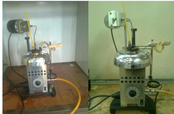
**Figure 4.6** Closed cup flash point.
