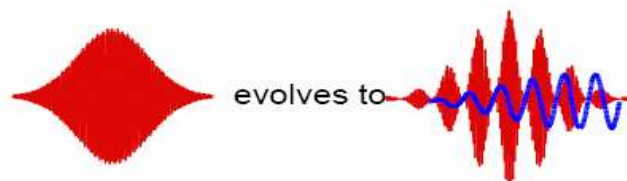
Figure (1-3) Plasma electron oscillations (blue line) as excited by Raman forward scattering (red line) in a plasma [10].
