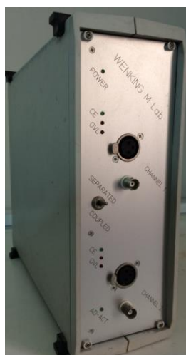
Figure (2.3): Front facing panel Potentiostat/Galvanostat.
