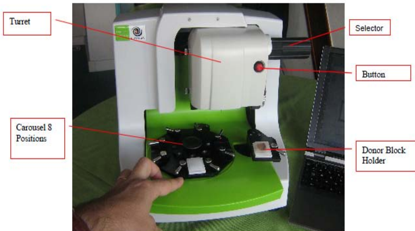
Figure (2-1) Minicore Tissue Microarrayer (Alphelys-TMA, Plaisir, France).
