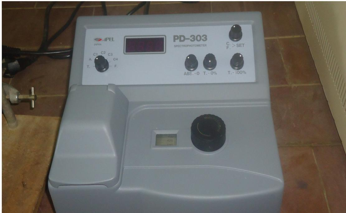
Image (2-7): Apel PD-303 single beam visible spectrophotometer
