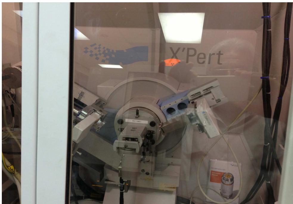
Image (2-5): Pananalytical Philips diffractometer (Georgia Institute of Technology, Atlanta, GA, USA)
