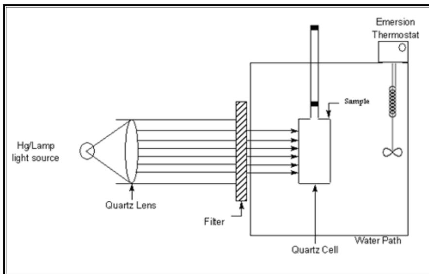
Figure (2.1): (a) Photolysis apparatus set up.
