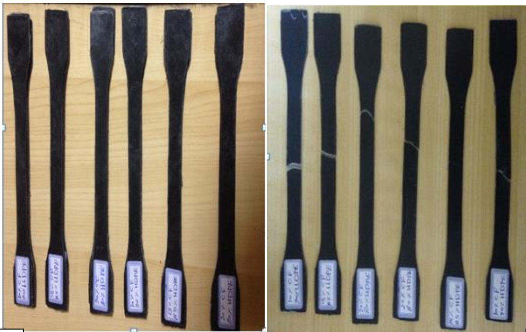
figure 4-9 Standard Specimens of Composite Material for Tensile Test
