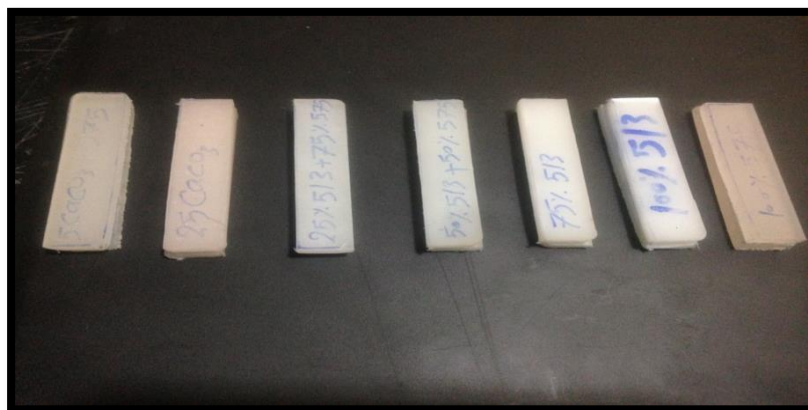
figure 4-12 Impact specimens of polypropylene blends
