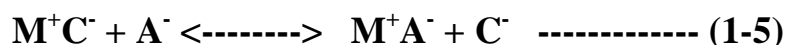
Figure (1-1) The principle of retention by exchange of anions in anion-exchange chromatography.
