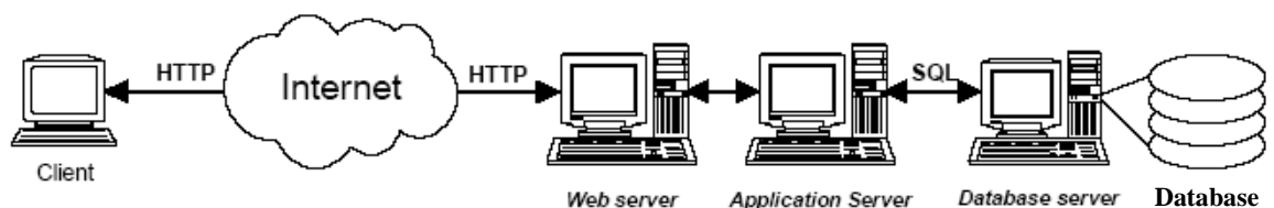
Figure (3.2) Typical Configuration of Dynamic Content Website
