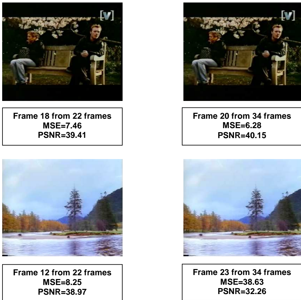
Figure (4.12) Some of the reconstructed video frames at different values of GOP size (using MOTS method).
