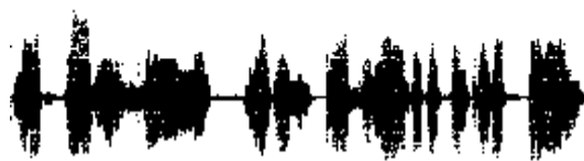
Quantized signal with quantization step = 2
