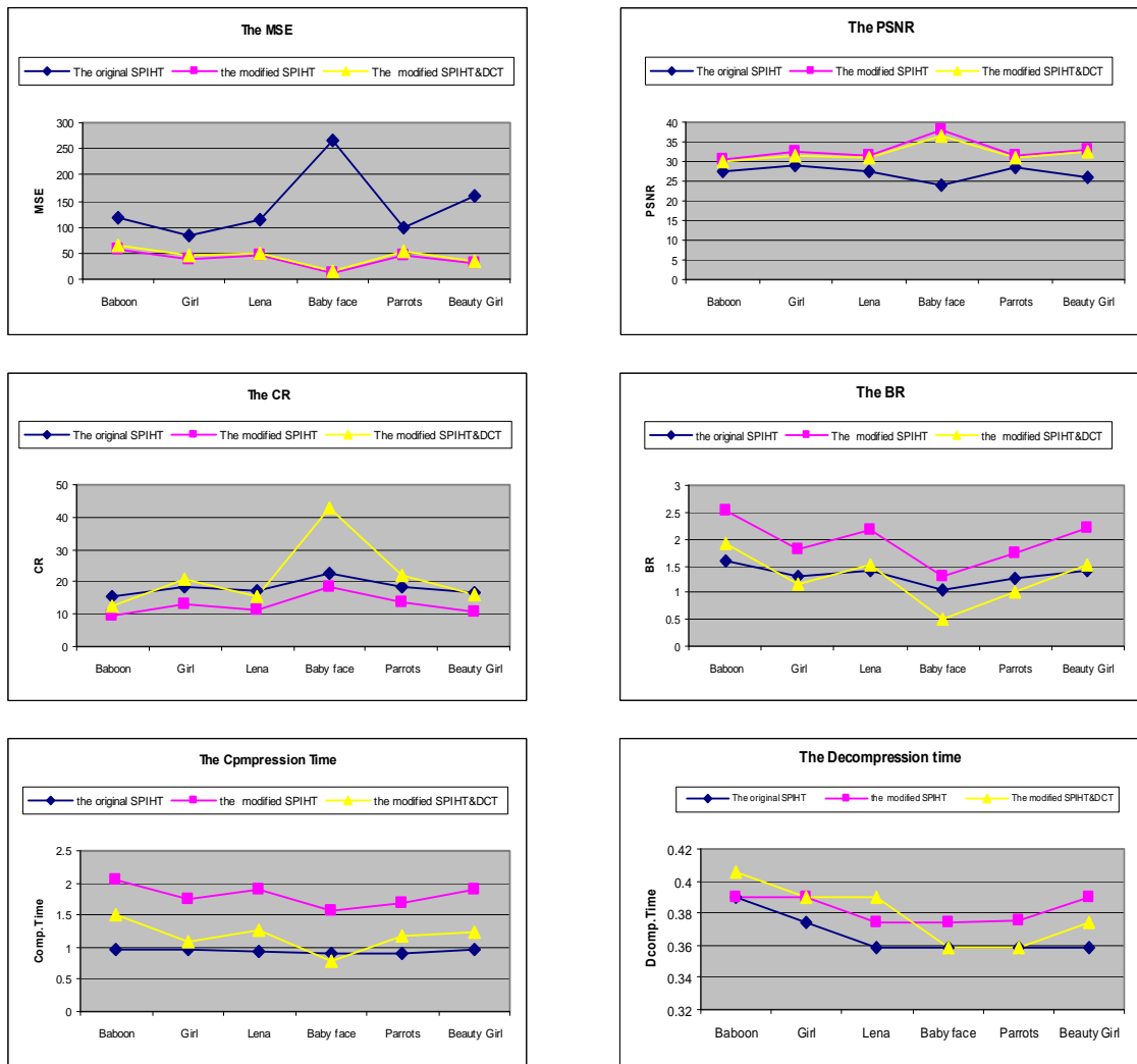
Figure (4.10) the differences between the results of the Original, Modified SPIHT and Modified SPIHT with DCT&RLE methods.
