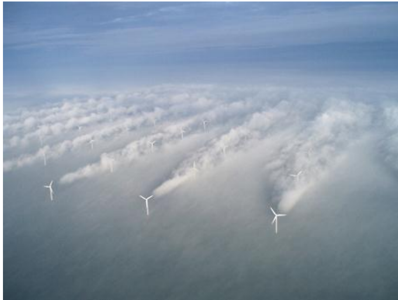
Fig. 2.27 Wake effects from neighbouring wind turbines, [Gau].
