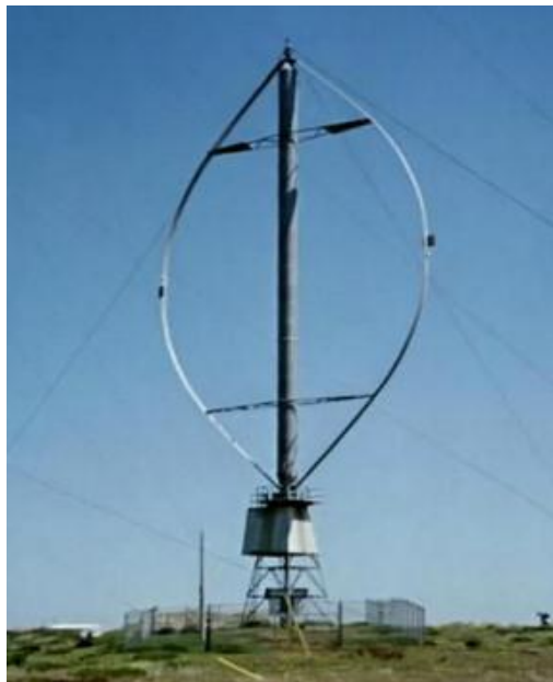
Fig. 2.18 Vertical axis wind turbine (VAWT), [Min09].
