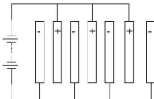
Figure 2.5 Monopolar connection of electrodes in electrochemical reactors
