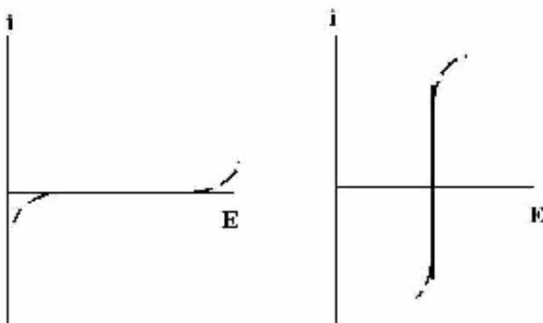
**Figure 2.3** Polarization of electrodes: Ideal polarization electrode to the left and to the right ideal nonpolarization electrode [11]
