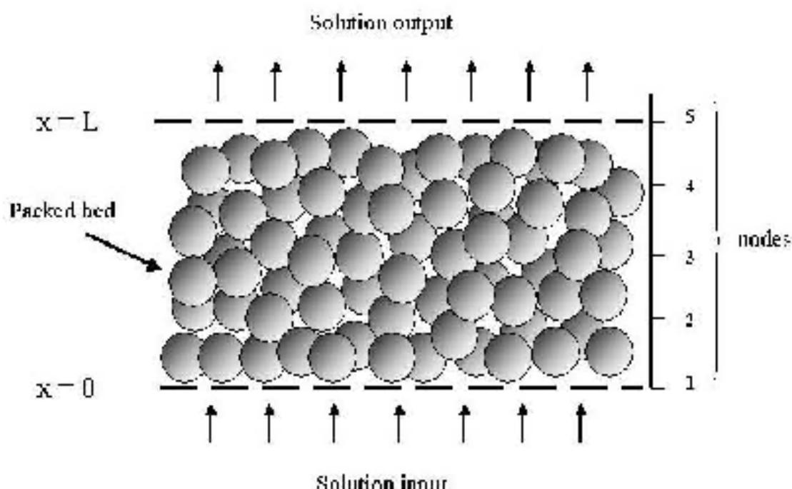
**Fig. 3.3** Schematic diagram of the working electrode
