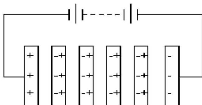
Figure 2.6 Bipolar connection of electrodes in electrochemical reactors [15]
