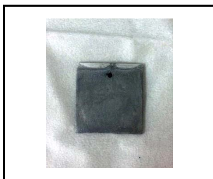
Figure (3-18): Photograph of Al-deposit on pure Mg sample in aluminum chloride/urea IL
