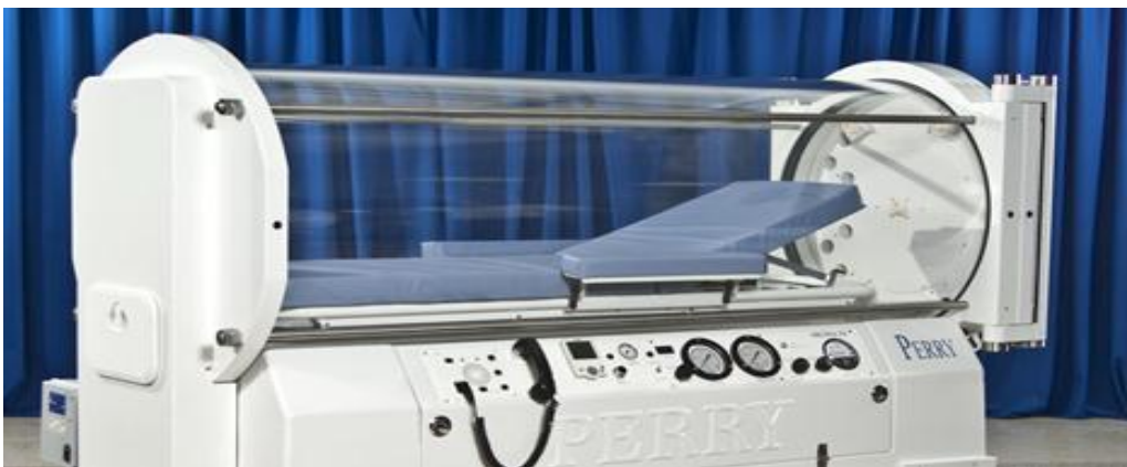
Figure(3.3): A hyperbaric chamber machine used to provide oxygen therapy to the patients.
