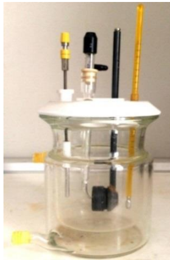
Figure (2-4): Corrosion cell set-up.
