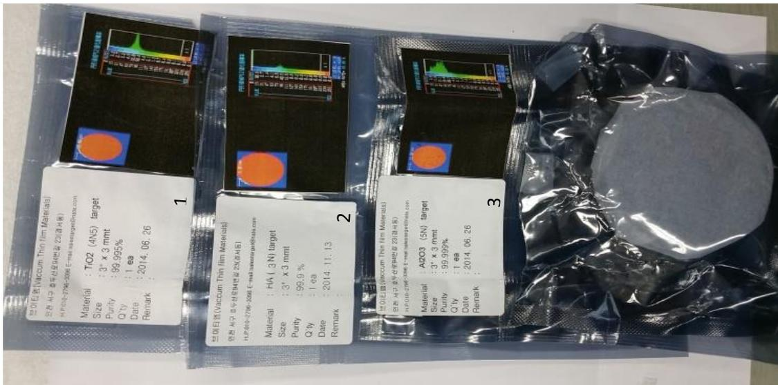
Figure 3.6: Targets ( $\text{TiO}_2$ , HA,  $\text{Al}_2\text{O}_3$ )
