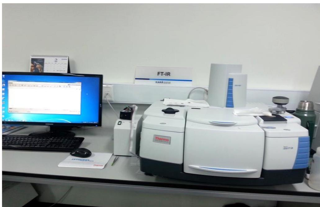
Figure 3.12: Fourier Transform Infrared Spectrometer (FTIR)
