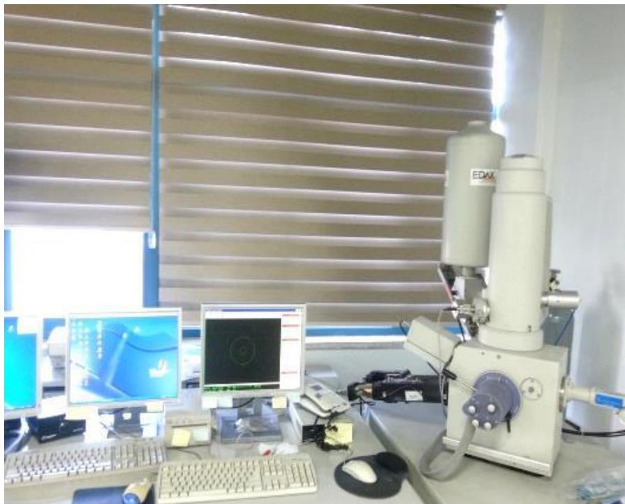
**Figure 3.9: Energy Dispersive X-ray Spectroscopy (EDS)**
