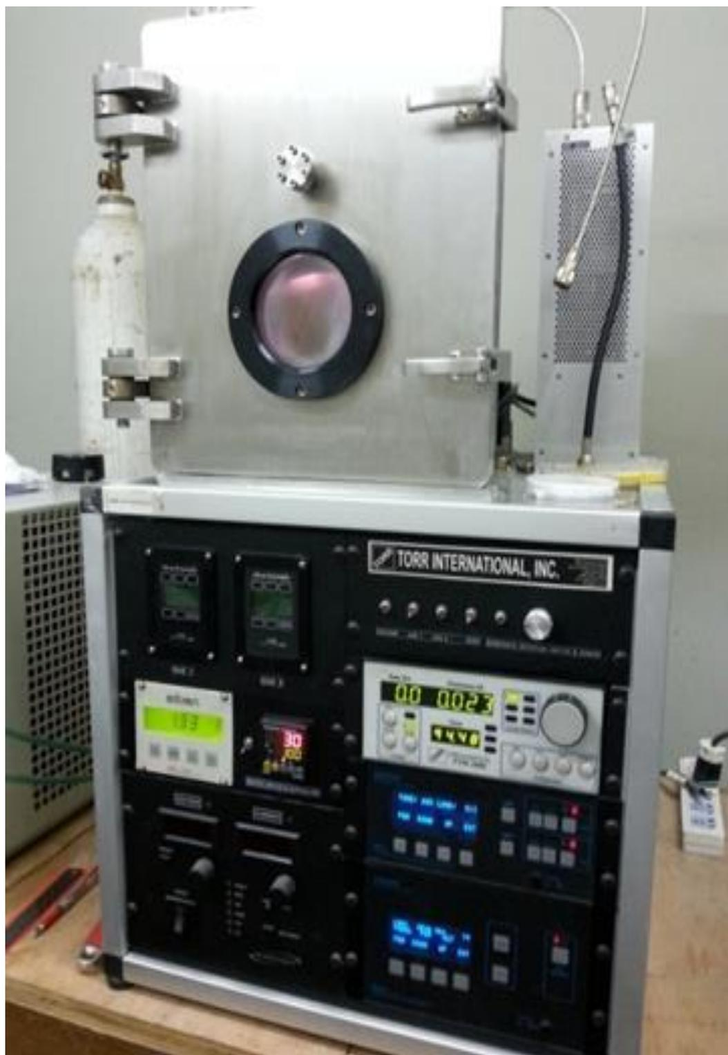
Figure 3.2 :RF magnetron sputtering system
