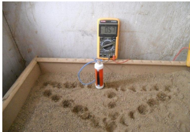
Figure 3-16 Set up potential contours measurements for anode in dry soil of position 20cm away from pipe.
