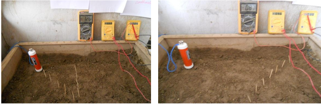
Figure 3-19 Set up potential contours measurements procedure of moisture soil
