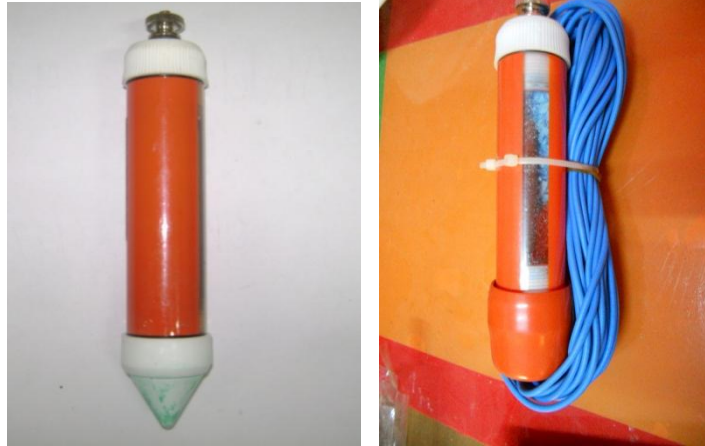
Figure 2-8 Copper/copper sulfate electrode
