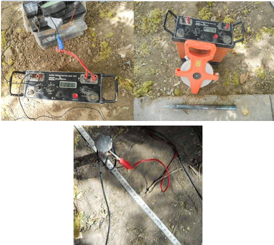
Figure 3-5 Soil resistivity measurement.
