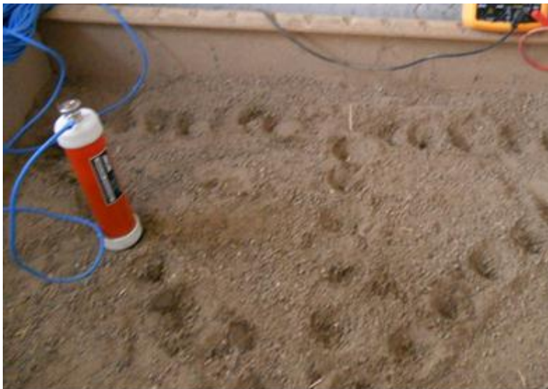
Figure 3-9 Copper-copper sulfate electrode
