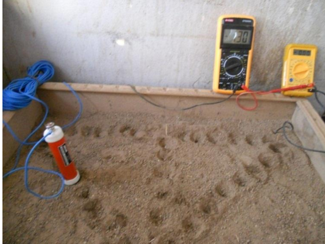
Figure 3-15 Set up potential contours measurements for anode in dry soil of position 30cm away from pipe.
