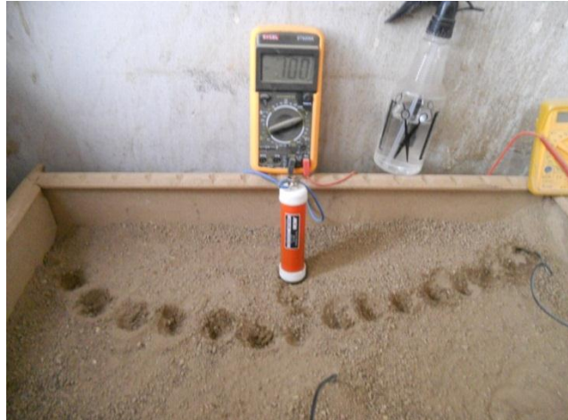
Figure3-17 Set up potential contours measurements for anode in dry soil of position 10cm away from pipe.
