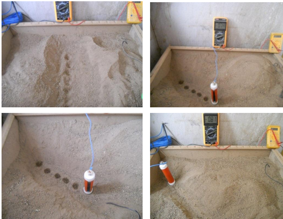
Figure3-18 Set up potential contours measurements procedure for different electrode depth Position.
