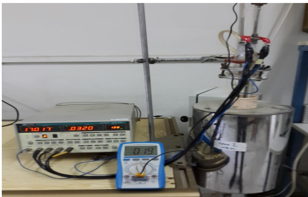
Fig. 2.2: The setup of dielectric measurement
