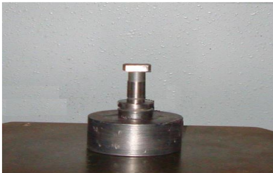
Fig. 2.1: The die used for pressing the powders.
